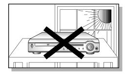
During thunderstorms, disconnect the main plug from the socket. Main voltage peaks due to lightning could damage the unit. Do not expose the unit to direct sun radiation or other heat sources.
